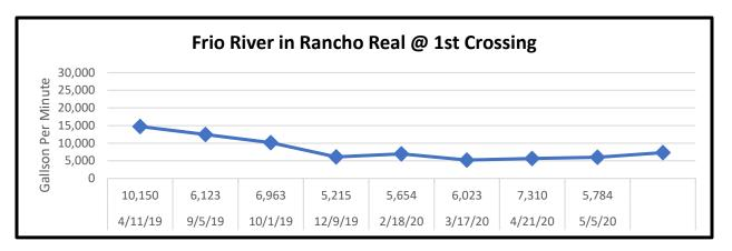
On Ranch Road 336 North of Leakey is Kent Creek which flows into the West Prong of the Frio River. This crossing showed a decrease in flow from 1,514 gpm to 201 gpm. Further north on RR 336 in Rancho Real, the 1<sup>st</sup> crossing of the West Prong of the Frio River recorded a decrease in flow of 7,310 gpm to 5,784 gpm. Both crossing measurements were taken on May 5, 2020, and both continue to have some debris and gravel impeding flow.
