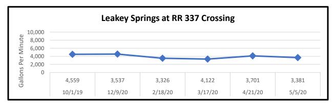
On <u>May 5, 2020</u>, east on Ranch Road 337 and past the cemetery is the serene Leakey Springs tributary that flows into the Frio River. This crossing measurement showed a flow of 3,701 gpm in April and now flows at 3,381 gpm.
