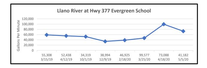
Both Llano River crossings in northern Edwards County were taken on May 5, 2020. As you can see, there is a decrease in flow for both Telegraph and Evergreen crossings. For the crossing at Telegraph on Highway 377, the South Llano River had a flow of 66,239 gpm in April and now has a flow of 51,572 gpm. At the Evergreen School crossing, the flow in April was 73,088 gpm and the flow is now 41,182 gpm.
